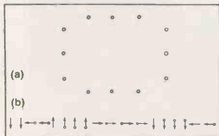
Figure 1. In order to draw the shape (a) by conventional means, you have to convert it to a set of vectors (b) which are then plotted.
